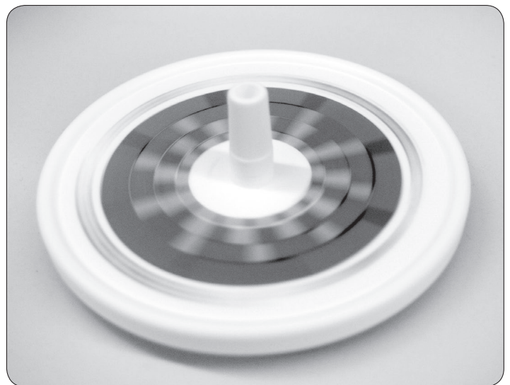
FLICKER CHECKER SHOWING A MAGNETIC BALLAST
